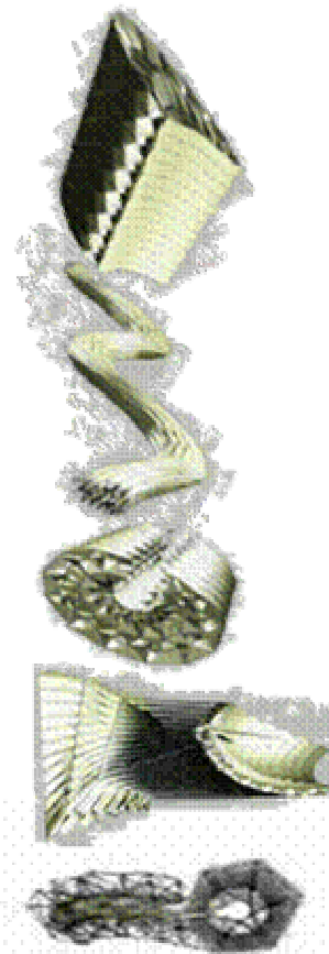
Figure 17 ANTS Continuous structure proposed for LARA. Transformations from flattened form to snakelike and rolling forms and finally to antenna and beacon forms.
